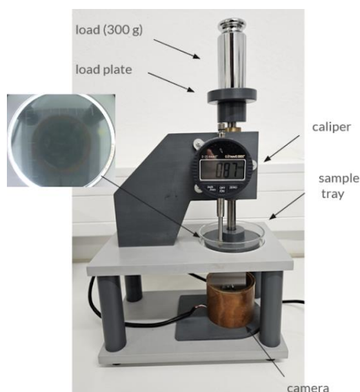
Fig. 1. "Sandwich test" device.
